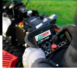
The RC-1000s comes with two rechargeable batteries that can be charged directly on the machine during use, ensuring uninterrupted operation. The ergonomic remote control gives you control of the machine from up to 150 metres away.
